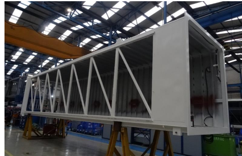
Figure 2-10 - Prefabricated modular Fixed Links
